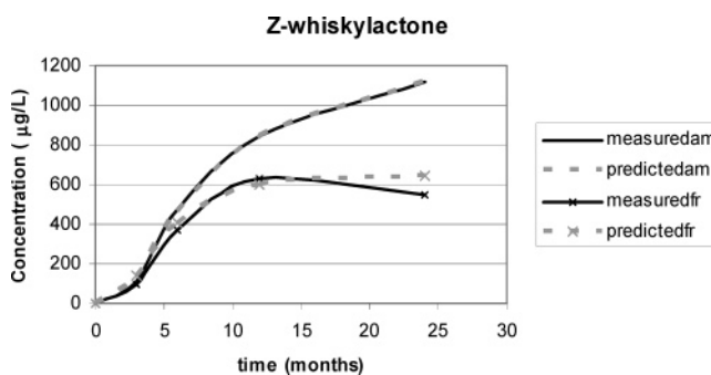
Figure 5. Fitting of experimental data "concentration of Z-whiskeylactone extracted" versus time (a single extraction) with eq 13 for two different sets of barrels (American and French). Original data are from ref 1. For American oak K_1 = 1200 \mu\text{g/L} and K_2 = 0.12 \mu\text{g/L} . For French oak K_1 = 650 \mu\text{g/L} and K_2 = 0.25 \mu\text{g/L} .
